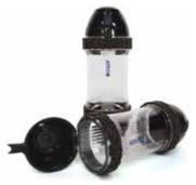
contents and latching it shut with the other, eliminating the potential for unlatched transport and overstuffing of contents that can lead to tube system failure. The high-impact polycarbonate body is capped with energy-absorbent rubber ends for strength, quiet delivery, and vertical standing. A variety of carrier options are available, with colored ends and a clear body for easy content identification, and are compatible with most 6-inch tube systems.
