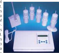
bed, sending an alert message to staff so they can ensure the resident is not in need. QuietCare also remotely alerts caregivers to potential medical emergencies, such as possible bathroom falls, thereby enabling an early intervention. The system also provides alerts when the room temperature is dangerously high or low.
