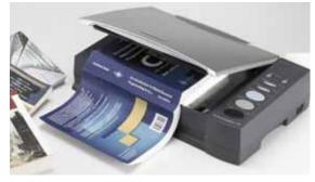
allow the scanner to copy and "read" the documents scanned. The user places a book or document on the screen, presses a button, and the Book Reader transforms printed words into audio output, which can be saved in MP3 format for future access. The Book Reader is bundled with ScanSoft's RealSpeak Solo 4 to provide lifelike voices.
