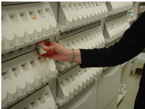
PharmASSIST cabinets in UNC Healthcare's outpatient pharmacies store and dispense 100 common medications.
