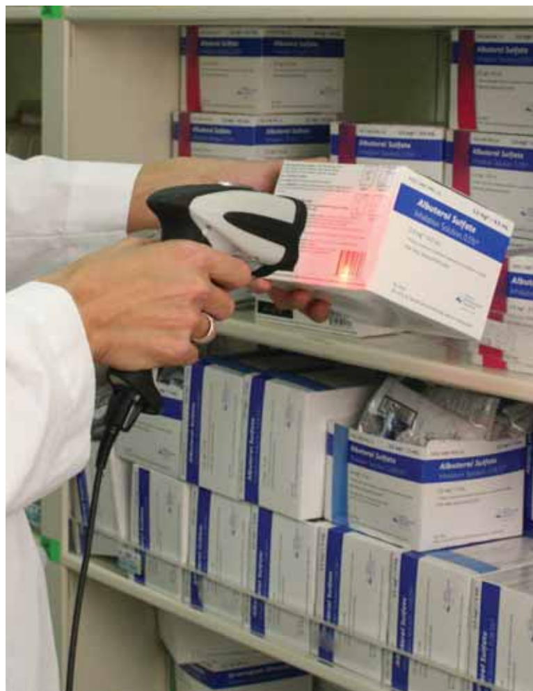
Purchasing bar code imagers, which can read both linear and the increasingly prevalent two-dimensional bar codes on medication packaging, can help to "future proof" your facility's BCMA program.
