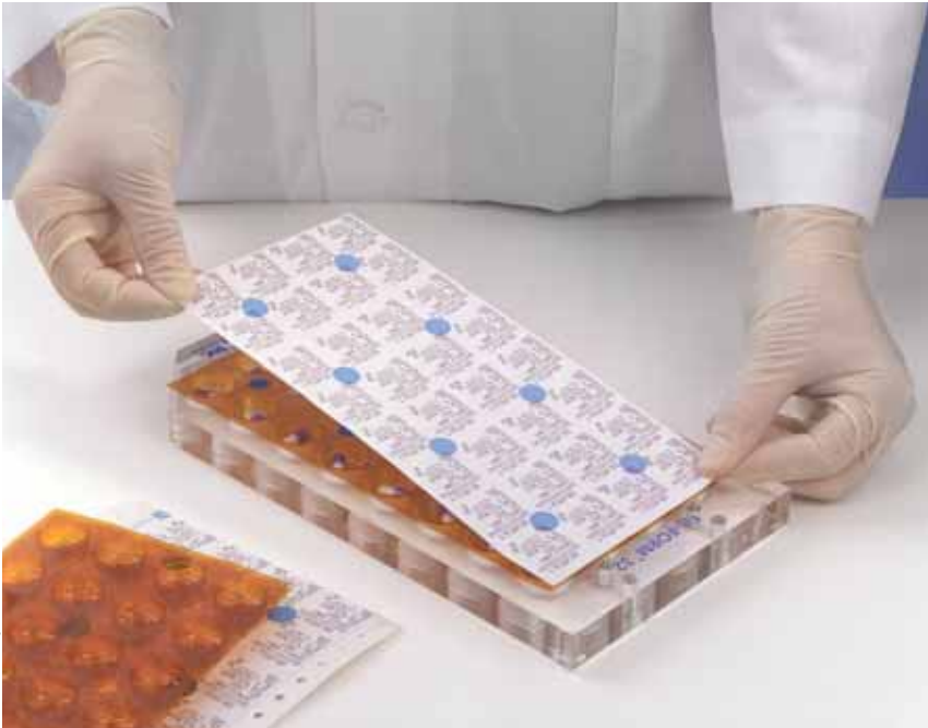
In addition to automated systems, manual systems for packaging medications in punch cards, such as this one from Medi-Dose, are also available.
