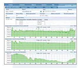
system consists of a wireless temperature module, which serves as the primary measuring device and collects data from the refrigeration unit; a wireless environment manager, which receives data from the wireless temperature modules and serves as a network access point; and the Web-based INM software platform, through which users can view temperature logs, daily reports, and alerts.
