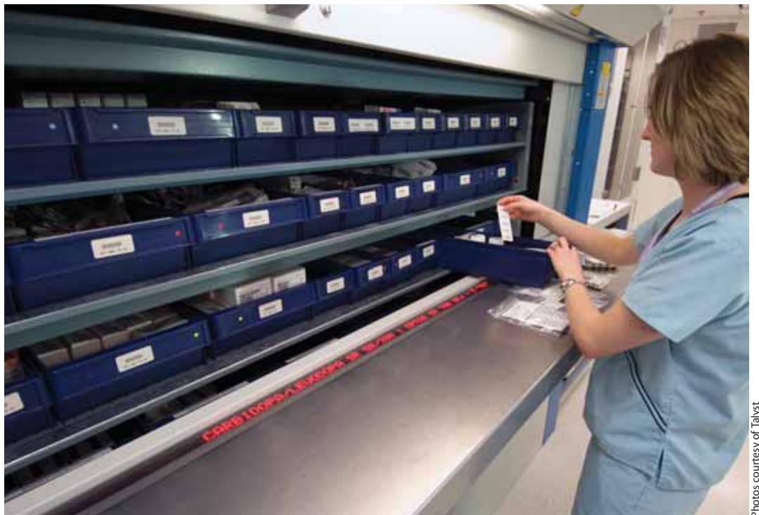
In the central pharmacy, the carousel/packager and its accompanying software enable a distribution solution that verifies bar codes as medications are stocked and again as they are distributed.
